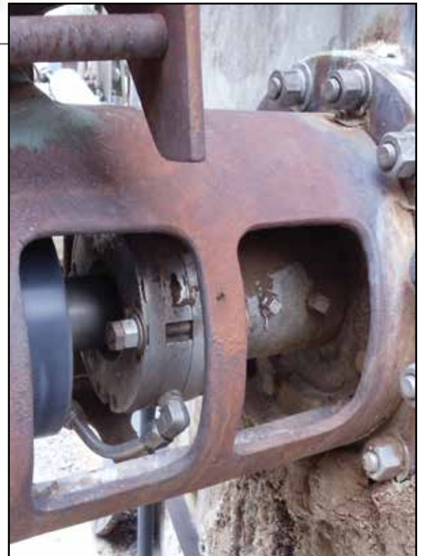
A stainless steel Air Mizer shaft seal installed on a side entry agitator eliminates product waste and contamination.
