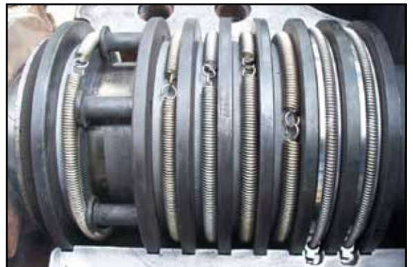
Typically, two Sentinel FBS's are installed in each gland box to provide superior sealing protection.
